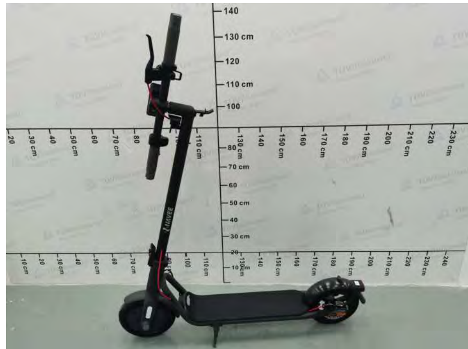
Version 04: the foldable handlebar, with direction indicator
