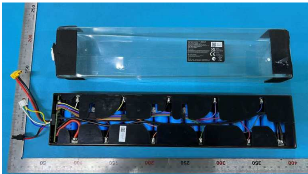
Picture 4. Internal view 1 of Battery
