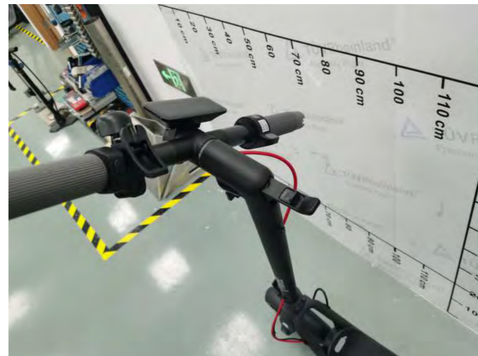
Version 04: the foldable handlebar, with direction indicator
