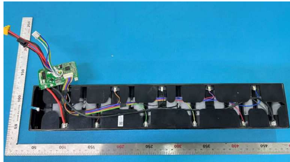
Picture 5. Internal view 2 of Battery
